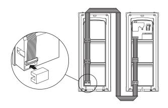
Supplied as standard with the audio and video speaker module, is a closing accessory with connector. The accessory must be fitted in the last pushbutton module of the entrance panel, after connecting the modules to each other using the multicables.
