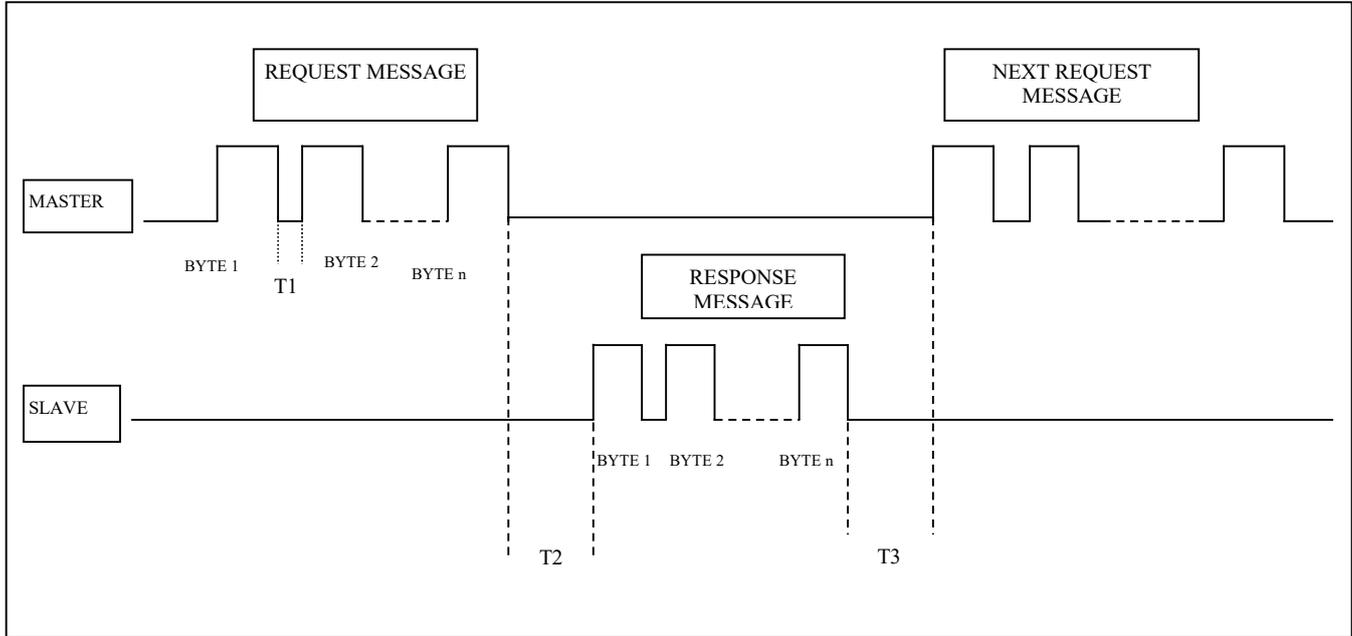
**Be careful :** among the setup parameters there is a timeout value that may be programmed. This is the inter-characters timeout and implicitly is the timeout to detect the end of a message. The value of 20 msec is suggested to keep compatibility with older IME devices. The minimum value is 3 msec.
