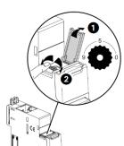
. Marked from 0 to 9 in order to locally define the Modbus address to Nemo SX modules In this system the Modbus address of a Nemo SX Nemo SX module device or group of modules (several functions) is obtained considering the address of the interface Modbus/Nemo SX Interface as tenth and the address of a device or group of function as unit (e.g. Interface address  $1=10 \rightarrow \text{address}$  of module n° 5=Modbus address 15)
