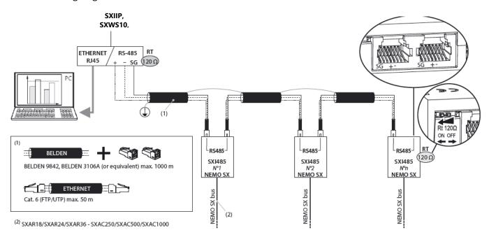
Note: it is not necessary to dedicate a RS485 / IP gateway for the Nemo SX system. It is possible to mix several RS485 devices.
