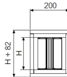
Dimension H changes with the ratings and it is specified in Table A (busbar dimension vs ratings), in appendix of the technical sheet
