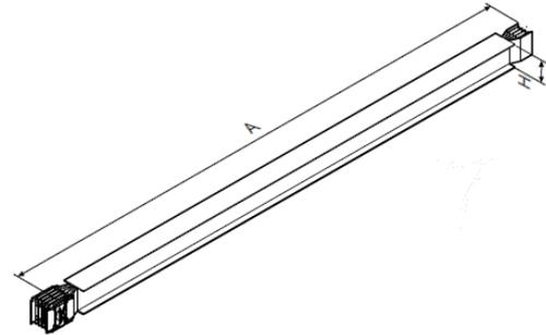
Dimension H changes with the ratings and it is specified in Table A (busbar dimension vs ratings), in appendix of the technical sheet
