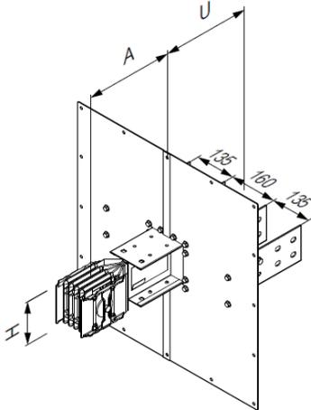
Dimension H changes with the ratings and it is specified in Table A (busbar dimension vs ratings), in appendix of the technical sheet
