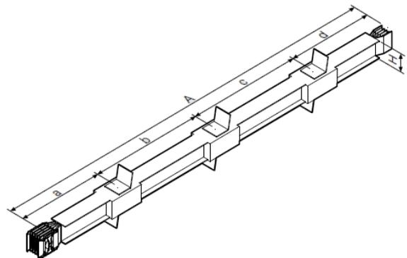
Dimension H changes with the ratings and it is specified in Table A (busbar dimension vs ratings), in appendix of the technical sheet
