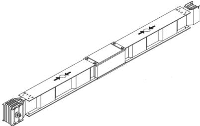
The length is 1.5 m and Dimension H changes with the ratings and it is specified in Table A (busbar dimension vs ratings), in appendix of the technical sheet
