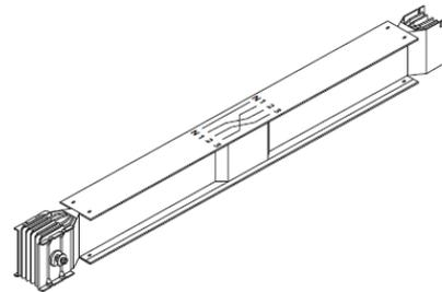
The length is 1.2 m and dimension H changes with the ratings and it is specified in Table A (busbar dimension vs ratings), in appendix of the technical sheet
