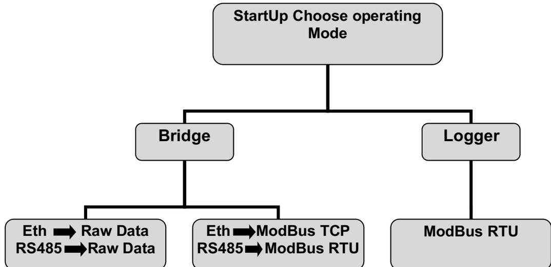
**Bridge with Raw Data** : any protocol can be transported over ETHERNET without any further manipulation. Modbus over TCP is the way to carry the Modbus RTU protocol as if it were transmitted on a normal RS485 line
